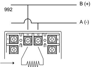
Install 121 ohm resistor on last control in chain.
