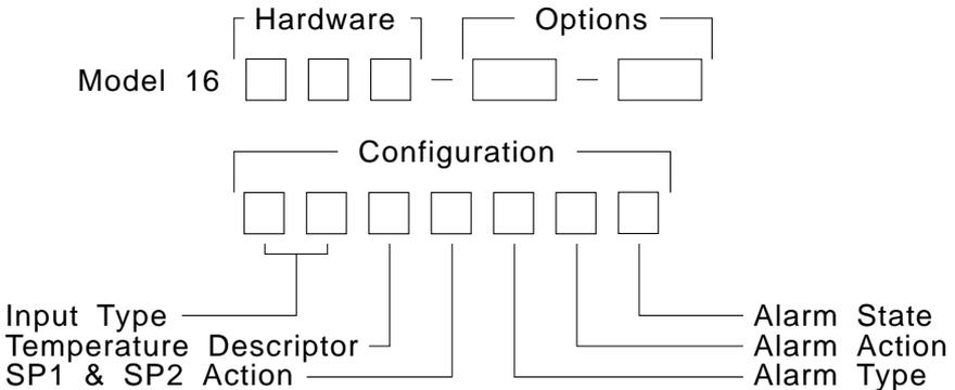
The Hardware configuration code **must not** be changed as it defines the hardware for the specific instrument. All other configuration may be altered if necessary. It is important that the codes be correctly entered in order for the instrument to function properly. If an invalid code number is entered for a particular configuration item, it will not be accepted and the old configuration code will be retained.
