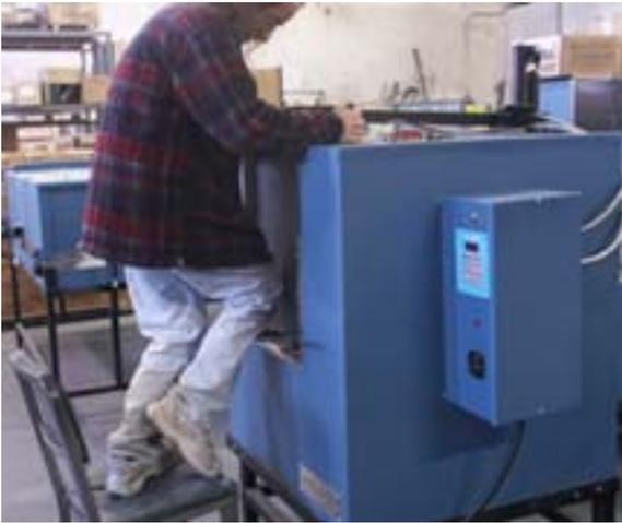
Place your knee firmly in the center of the lower part of the door and shove it flat up against the port casting. Once again, there should be no gap between the door and the port. You may need to force it a little by jiggling the top, but look down from the top and make sure its closed.
